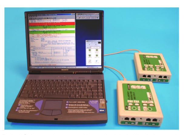
The Acacia Clarinet-system is a compact modular protocol analysis, simulation, development and conformance test system for ISDN, V5, QSIG, IP, SS7 and ATM.
