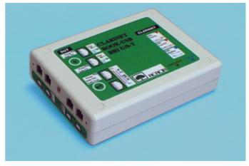
The software, control and operation is exactly the same as the SCSI pods for ISDN detailed in the following pages. The pod has a built in bit error rate tester, codec, digital port and handset port (handset supplied
