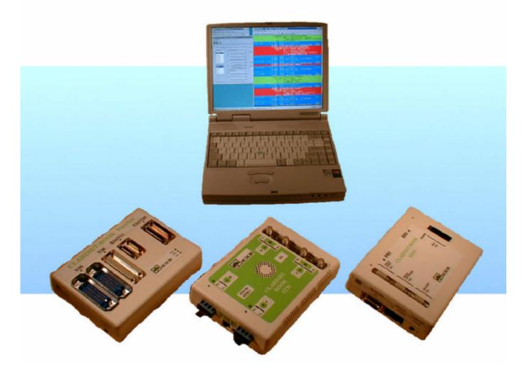
Clarinet-system developed by ACACIA is a powerful tool for testing protocols on ATM, WAN and LAN networks. The Clarinet-Book can be connected to a Desktop-PC or Notebook running under Windows<sup>™</sup>95, Windows<sup>™</sup>98 or Windows<sup>™</sup>NT 4.0.
